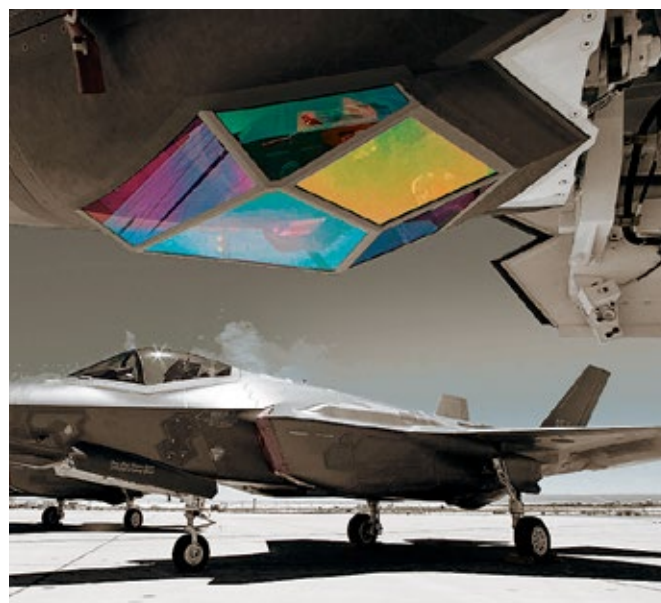
Industrial sapphires grown by research scientist Drew Haven '13 PhD are used to protect sensors within military aircraft. Courtesy Lockheed Martin
